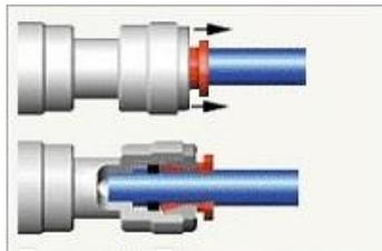
After tightening, pull both fittings and tubes to check if the tube does not come off. At this time, the clip will come out slightly as shown in the figure and will hold the tube so that it will not come off.
