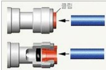
Insert the tube into the insertion slot with the fitting clip.
