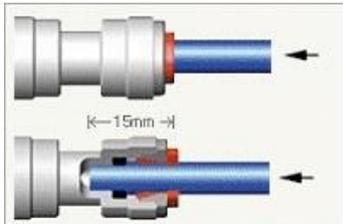
Push the tube all the way into the fitting to finish the tightening.
